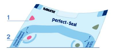
Class 1 external process indicators (that are located outside the instrument area ) are intended to indicate that the unit has been directly exposed to the sterilization process and to distinguish between process and unprocessed units.
